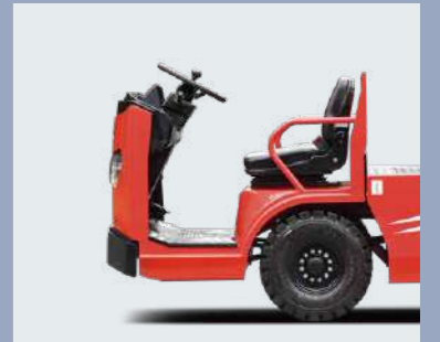
Full suspension operating platform, vibration is reduced, noise is isolated
